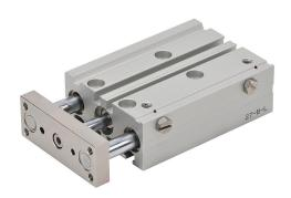
NITRA pneumatic cylinder, dual guide rod, 12mm bore, 6mm rod diameter, 50mm stroke, double acting, magnetic piston, universal mount.
