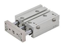
NITRA pneumatic cylinder, dual guide rod, 12mm bore, 6mm rod diameter, 40mm stroke, double acting, magnetic piston, universal mount.
