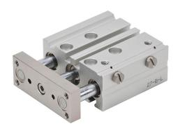
NITRA pneumatic cylinder, dual guide rod, 12mm bore, 6mm rod diameter, 25mm stroke, double acting, magnetic piston, universal mount.
