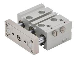
NITRA pneumatic cylinder, dual guide rod, 12mm bore, 6mm rod diameter, 10mm stroke, double acting, magnetic piston, universal mount.
