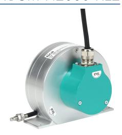
Lika Electronic DWI series incremental (quadrature) linear draw wire encoder, 5-30 VDC, universal (line driver or NPN/PNP open collector) output, medium duty, 0.025mm/count, 16.4ft/5m draw wire, IP65, 6.5ft/2m cable length, radial exit, pigtail.
