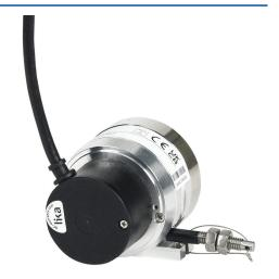
Lika Electronic DWI series incremental (quadrature) linear draw wire encoder, 5-30 VDC, universal (line driver or NPN/PNP open collector) output, light duty, 0.05mm/count, 6.5ft/2m draw wire, IP64, 6.5ft/2m cable length, radial exit, pigtail.
