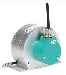
Lika Electronic DWI series incremental (quadrature) linear draw wire encoder, 5-30 VDC, universal (line driver or NPN/PNP open collector) output, medium duty, 0.025mm/count, 32.8ft/10m draw wire, IP65, 6.5ft/2m cable length, radial exit, pigtail.
