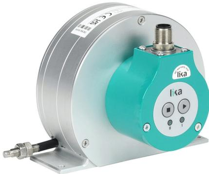
Lika Electronic DWA series programmable analog linear draw wire encoder, 13-30 VDC, 4-20 mA output, medium duty, 0.366  $\mu$ A/step, 16.4ft/5m draw wire, IP65, radial exit, 5-pin M12 female A-coded.
