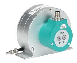
Lika Electronic DWA series programmable analog linear draw wire encoder, 13-30 VDC, 0-10 VDC output, medium duty, 0.153 mV/ step, 16.4ft/5m draw wire, IP65, radial exit, 5-pin M12 female Acoded.
