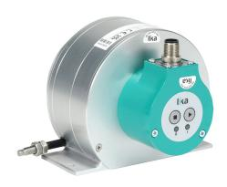
Lika Electronic DWA series programmable analog linear draw wire encoder, 13-30 VDC, 4-20 mA output, medium duty, 0.366  $\mu$ A/ step, 32.8ft/10m draw wire, IP65, radial exit, 5-pin M12 female A-coded.
