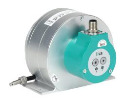
Lika Electronic DWA series programmable analog linear draw wire encoder, 13-30 VDC, 0-10 VDC output, medium duty, 0.153 mV/ step, 32.8ft/10m draw wire, IP65, radial exit, 5-pin M12 female A-coded.
