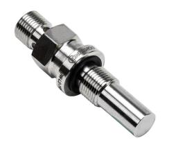
Contrinex inductive proximity sensor, tubular, 12mm diameter x 61mm body, 304 stainless steel housing, PNP, N.O., 1.5mm sensing distance, flush, 850 Hz switching frequency, IP68 IP69K, 4-pin M12 quick-disconnect.
