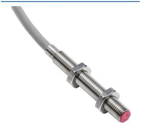
Contrinex inductive proximity sensor, tubular, 8mm diameter x 60mm body, 304 stainless steel housing, PNP, N.O., 2mm sensing distance, flush, 600 Hz switching frequency, IP67, pigtail.
