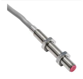
Contrinex inductive proximity sensor, tubular, 8mm diameter x 60mm body, 304 stainless steel housing, NPN, N.O., 2mm sensing distance, flush, 600 Hz switching frequency, IP67, pigtail.
