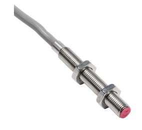
Contrinex inductive proximity sensor, tubular, 8mm diameter x 60mm body, 304 stainless steel housing, NPN, N.O., 2mm sensing distance, flush, 600 Hz switching frequency, IP67, pigtail.
