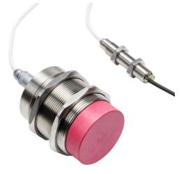
Contrinex inductive proximity sensor, tubular, 50mm diameter x 68mm body, 304 stainless steel housing, PNP, N.O., 25mm sensing distance, non-flush, 150 Hz switching frequency, IP67, pigtail.
