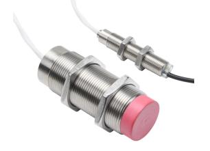
Contrinex inductive proximity sensor, tubular, 30mm diameter x 83mm body, 304 stainless steel housing, PNP, N.O., 15mm sensing distance, non-flush, 150 Hz switching frequency, IP67, pigtail.
