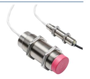
Contrinex inductive proximity sensor, tubular, 30mm diameter x 83mm body, 304 stainless steel housing, NPN, N.O., 15mm sensing distance, non-flush, 150 Hz switching frequency, IP67, pigtail.
