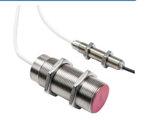
Contrinex inductive proximity sensor, tubular, 30mm diameter x 75mm body, 304 stainless steel housing, PNP, N.O., 10mm sensing distance, flush, 200 Hz switching frequency, IP67, pigtail.
