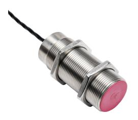
Contrinex inductive proximity sensor, tubular, 30mm diameter x 75mm body, 304 stainless steel housing, PNP, N.O., 10mm sensing distance, flush, 200 Hz switching frequency, IP67, pigtail.
