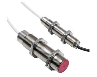
Contrinex inductive proximity sensor, tubular, 18mm diameter x 76mm body, 304 stainless steel housing, PNP, N.O., 5mm sensing distance, flush, 300 Hz switching frequency, IP67, pigtail.
