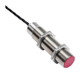
Contrinex inductive proximity sensor, tubular, 18mm diameter x 76mm body, 304 stainless steel housing, PNP, N.O., 5mm sensing distance, flush, 400 Hz switching frequency, IP67, pigtail.
