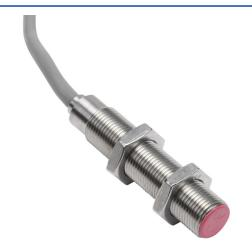
Contrinex inductive proximity sensor, tubular, 12mm diameter x 59mm body, 304 stainless steel housing, PNP, N.O., 3mm sensing distance, flush, 500 Hz switching frequency, IP67, pigtail.
