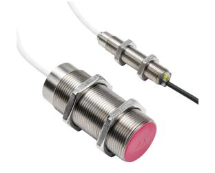
Contrinex inductive proximity sensor, tubular, 30mm diameter x 75mm body, 304 stainless steel housing, NPN, N.O., 10mm sensing distance, flush, 200 Hz switching frequency, IP67, pigtail.
