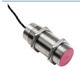
Contrinex inductive proximity sensor, tubular, 30mm diameter x 75mm body, 304 stainless steel housing, NPN, N.O., 10mm sensing distance, flush, 200 Hz switching frequency, IP67, pigtail.
