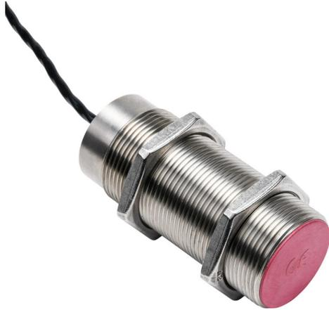
Contrinex inductive proximity sensor, tubular, 30mm diameter x 75mm body, 304 stainless steel housing, NPN, N.O., 10mm sensing distance, flush, 200 Hz switching frequency, IP67, pigtail.
