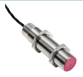
Contrinex inductive proximity sensor, tubular, 18mm diameter x 76mm body, 304 stainless steel housing, NPN, N.O., 5mm sensing distance, flush, 400 Hz switching frequency, IP67, pigtail.
