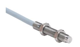
Contrinex inductive proximity sensor, tubular, 5mm diameter x 30mm body, stainless steel housing, PNP, N.O. output, 3mm sensing distance, non-flush, 1.2 kHz switching frequency, IP67, 3-pin M8 quick-disconnect.
