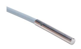
Contrinex inductive proximity sensor, tubular, 4mm diameter x 30mm body, stainless steel housing, PNP, N.O. output, 3mm sensing distance, non-flush, 1.2 kHz switching frequency, IP67, 3-pin M8 quick-disconnect.
