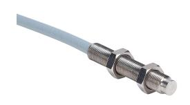
Contrinex inductive proximity sensor, tubular, 5mm diameter x 30mm body, stainless steel housing, NPN, N.O. output, 3mm sensing distance, non-flush, 1.2 kHz switching frequency, IP67, 3-pin M8 quick-disconnect.
