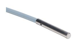
Contrinex inductive proximity sensor, tubular, 4mm diameter x 30mm body, stainless steel housing, NPN, N.O. output, 3mm sensing distance, non-flush, 1.2 kHz switching frequency, IP67, 3-pin M8 quick-disconnect.
