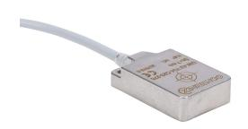
Contrinex inductive proximity sensor, rectangular, 32 x 20 x 8mm body, stainless steel housing, PNP, N.C. output, 7mm sensing distance, flush, 180 Hz switching frequency, IP68 IP69K, 3-pin M8 quick-disconnect.
