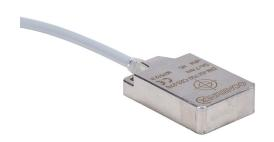
Contrinex inductive proximity sensor, rectangular, 32 x 20 x 8mm body, stainless steel housing, NPN, N.C. output, 7mm sensing distance, flush, 180 Hz switching frequency, IP68 IP69K, 3-pin M8 quick-disconnect.
