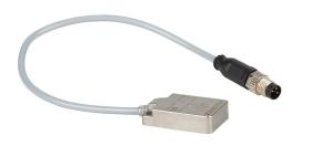
Contrinex inductive proximity sensor, rectangular, 32 x 20 x 8mm body, stainless steel housing, NPN, N.O. output, 7mm sensing distance, flush, 180 Hz switching frequency, IP68 IP69K, 3-pin M8 quick-disconnect.
