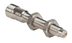
Contrinex inductive proximity sensor, tubular, 8mm diameter x 66mm body, stainless steel housing, PNP, N.C. output, 6mm sensing distance, non-flush, 700 Hz switching frequency, IP67 IP68, 4-pin M12 quick-disconnect.
