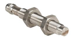
Contrinex inductive proximity sensor, tubular, 8mm diameter x 60mm body, stainless steel housing, PNP, N.C. output, 6mm sensing distance, non-flush, 700 Hz switching frequency, IP67 IP68, 3-pin M8 quick-disconnect.
