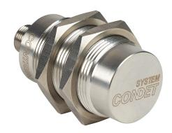
Contrinex inductive proximity sensor, tubular, 30mm diameter x 63.5mm body, stainless steel housing, PNP, N.C. output, 40mm sensing distance, non-flush, 90 Hz switching frequency, IP68 IP69K, 4-pin M12 quick-disconnect.
