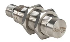
Contrinex inductive proximity sensor, tubular, 18mm diameter x 63.5mm body, stainless steel housing, PNP, N.C. output, 20mm sensing distance, non-flush, 200 Hz switching frequency, IP68 IP69K, 4-pin M12 quick-disconnect.
