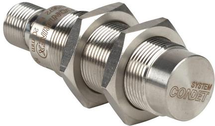
Contrinex inductive proximity sensor, tubular, 18mm diameter x 63.5mm body, stainless steel housing, PNP, N.C. output, 20mm sensing distance, non-flush, 200 Hz switching frequency, IP68 IP69K, 4-pin M12 quick-disconnect.
