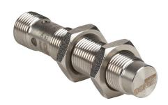
Contrinex inductive proximity sensor, tubular, 12mm diameter x 60mm body, stainless steel housing, PNP, N.C. output, 10mm sensing distance, non-flush, 400 Hz switching frequency, IP68 IP69K, 4-pin M12 quick-disconnect.
