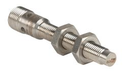
Contrinex inductive proximity sensor, tubular, 8mm diameter x 66mm body, stainless steel housing, PNP, N.O. output, 6mm sensing distance, non-flush, 700 Hz switching frequency, IP67 IP68, 4-pin M12 quick-disconnect.
