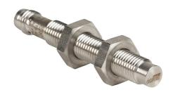
Contrinex inductive proximity sensor, tubular, 8mm diameter x 60mm body, stainless steel housing, PNP, N.O. output, 6mm sensing distance, non-flush, 700 Hz switching frequency, IP67 IP68, 3-pin M8 quick-disconnect.
