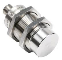
Contrinex inductive proximity sensor, tubular, 30mm diameter x 63.5mm body, 304 stainless steel housing, PNP, N.O., 12mm sensing distance, non-flush, 90 Hz switching frequency, IP68 IP69K, 4-pin M12 quick-disconnect.
