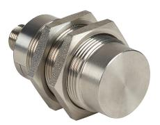
Contrinex inductive proximity sensor, tubular, 30mm diameter x 63.5mm body, stainless steel housing, PNP, N.O. output, 40mm sensing distance, non-flush, 90 Hz switching frequency, IP68 IP69K, 4-pin M12 quick-disconnect.
