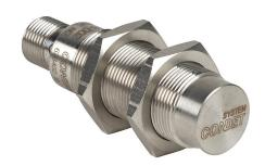
Contrinex inductive proximity sensor, tubular, 18mm diameter x 63.5mm body, stainless steel housing, PNP, N.O. output, 20mm sensing distance, non-flush, 200 Hz switching frequency, IP68 IP69K, 4-pin M12 quick-disconnect.
