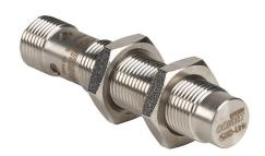
Contrinex inductive proximity sensor, tubular, 12mm diameter x 60mm body, stainless steel housing, PNP, N.O. output, 10mm sensing distance, non-flush, 400 Hz switching frequency, IP68 IP69K, 4-pin M12 quick-disconnect.
