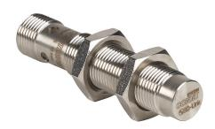
Contrinex inductive proximity sensor, tubular, 12mm diameter x 60mm body, stainless steel housing, PNP, N.O. output, 10mm sensing distance, non-flush, 400 Hz switching frequency, IP68 IP69K, 4-pin M12 quick-disconnect.
