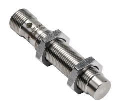
Contrinex inductive proximity sensor, tubular, 12mm diameter x 60mm, 304 stainless steel housing, PNP, N.O., 3mm sensing distance, non-flush, 400 Hz switching frequency, IP68 IP69K, 4-pin M12 quick-disconnect.
