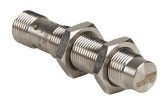
Contrinex inductive proximity sensor, tubular, 12mm diameter x 60mm body, stainless steel housing, NPN, N.C. output, 10mm sensing distance, non-flush, 400 Hz switching frequency, IP68 IP69K, 4-pin M12 quick-disconnect.
