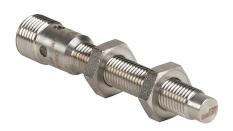
Contrinex inductive proximity sensor, tubular, 8mm diameter x 66mm body, stainless steel housing, NPN, N.O. output, 6mm sensing distance, non-flush, 700 Hz switching frequency, IP67 IP68, 4-pin M12 quick-disconnect.
