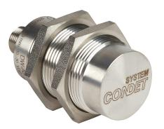
Contrinex inductive proximity sensor, tubular, 30mm diameter x 63.5mm body, stainless steel housing, NPN, N.O. output, 40mm sensing distance, non-flush, 90 Hz switching frequency, IP68 IP69K, 4-pin M12 quick-disconnect.
