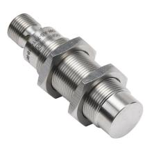
Contrinex inductive proximity sensor, tubular, 18mm diameter x 63.5mm body, 304 stainless steel housing, NPN, N.O., 5mm sensing distance, non-flush, 200 Hz switching frequency, IP68 IP69K, 4-pin M12 quick-disconnect.
