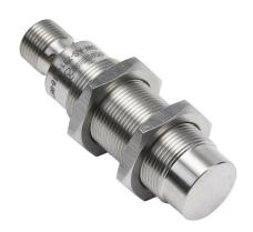
Contrinex inductive proximity sensor, tubular, 18mm diameter x 63.5mm body, 304 stainless steel housing, NPN, N.O., 5mm sensing distance, non-flush, 200 Hz switching frequency, IP68 IP69K, 4-pin M12 quick-disconnect.
