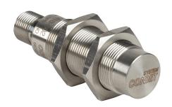
Contrinex inductive proximity sensor, tubular, 18mm diameter x 63.5mm body, stainless steel housing, NPN, N.O. output, 20mm sensing distance, non-flush, 200 Hz switching frequency, IP68 IP69K, 4-pin M12 quick-disconnect.
