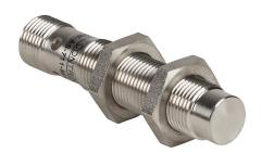
Contrinex inductive proximity sensor, tubular, 12mm diameter x 60mm body, stainless steel housing, NPN, N.O. output, 10mm sensing distance, non-flush, 400 Hz switching frequency, IP68 IP69K, 4-pin M12 quick-disconnect.
